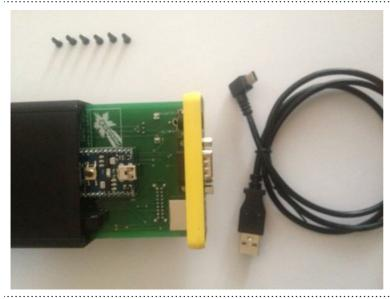
Slide the assembly out until you can see the spark logo on the underneath, at which point you should be able to locate the mini-USB socket on the end of the blue board.
