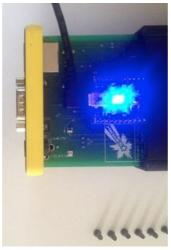
A blue light should appear on connecting to the computer's USB (the controller's power supply is not needed to access the USB drive).
