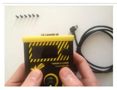
If the internal assembly does not readily slide out, try this alternative. Holding the body of the controller in your hands, use your thumbs to push along the top plate of the controller, so that it slides out along the controller's long axis.
