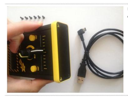
Remove the two screws at the top corners of the other, blank end-plate.
